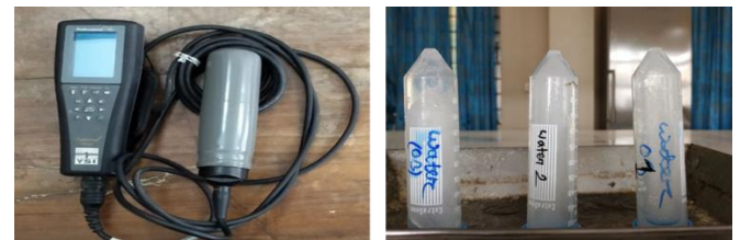
Figure 2. Portable water quality measuring kit (YSI ProDSS Multi-Parameter) and water sample preservation
