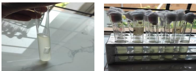
Figure 5: Photograph showing gas bubble in Durham's tube during Total Coliform Count (TCC).
